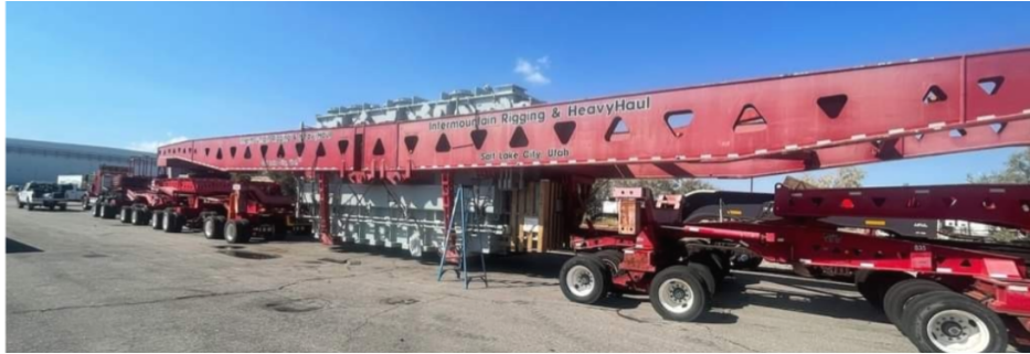
▲ Sedan Chair Type Transportation of 345kV 700MVA Transformer
