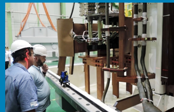
▲Returning of a transformer to the factory after a short-circuit test and visual inspection of the core by a KEMA technician
